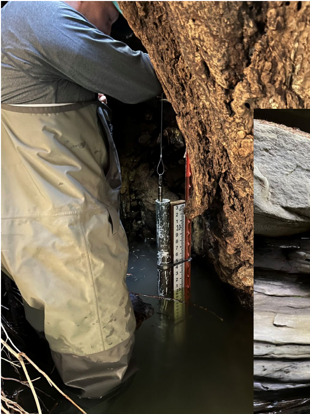
1. Data logger installed
